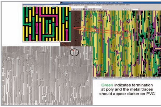
Passive Voltage Contrast (PVC) Checker identifies suspect vias or metal traces
